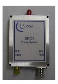
The SPGU splitter is an unusual high performance splitter designed particularly for satellite and GPS use. It is unusual in that it has one 750hm output and one 50 ohm output.
