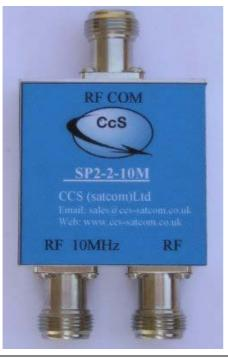
The SP2-2-10M is a high performance combiner splitter with a 10MHz and DC path designed particularly for VSAT use. The case is machined from Aluminium alloy and has a Nickel plated finish. Either N type or SMA connectors can be specified.
